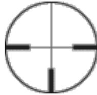
The most common and simplest reticles are the German #4 and the German #1. You'll see these reticles with thick right, bottom, and left (3, 6, and 9 o'clock) cross hairs that taper off towards the center in the original style or with a dot in the center. Sometimes it may or may not have a 12 o'clock/top cross hair.
