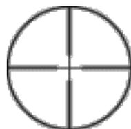
It's simple, uncluttered, and is considered the all-purpose reticle. The thicker posts of the four cross hairs will thin out to draw the eye to the center.
